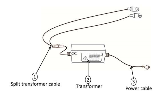
Step4: Plug transformer cables into sockets at back of sofa.
